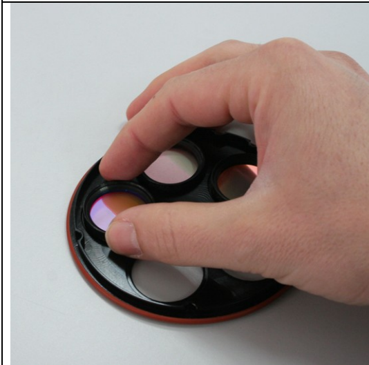
Install filters on disk
