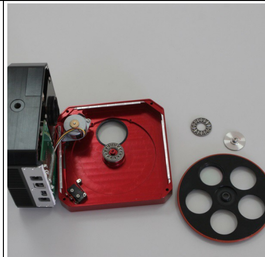
Remove the bearing by turning disk upside down. Parts should look as above.
