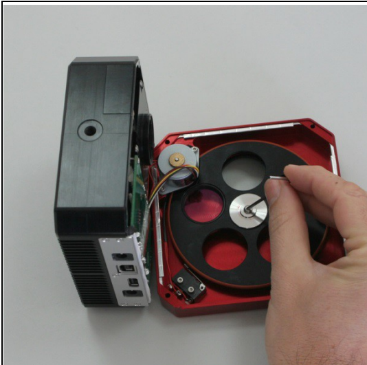
Unscrew the central holding screw.
